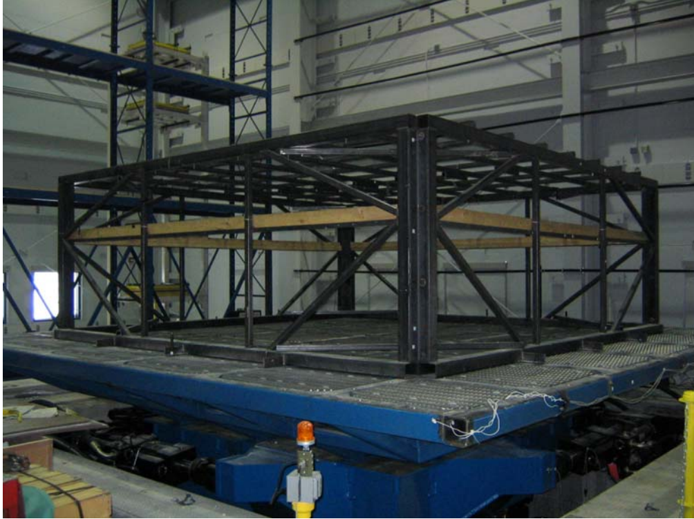
Figure 2.4 Test frame mounted on the shaking table at the University at Buffalo
